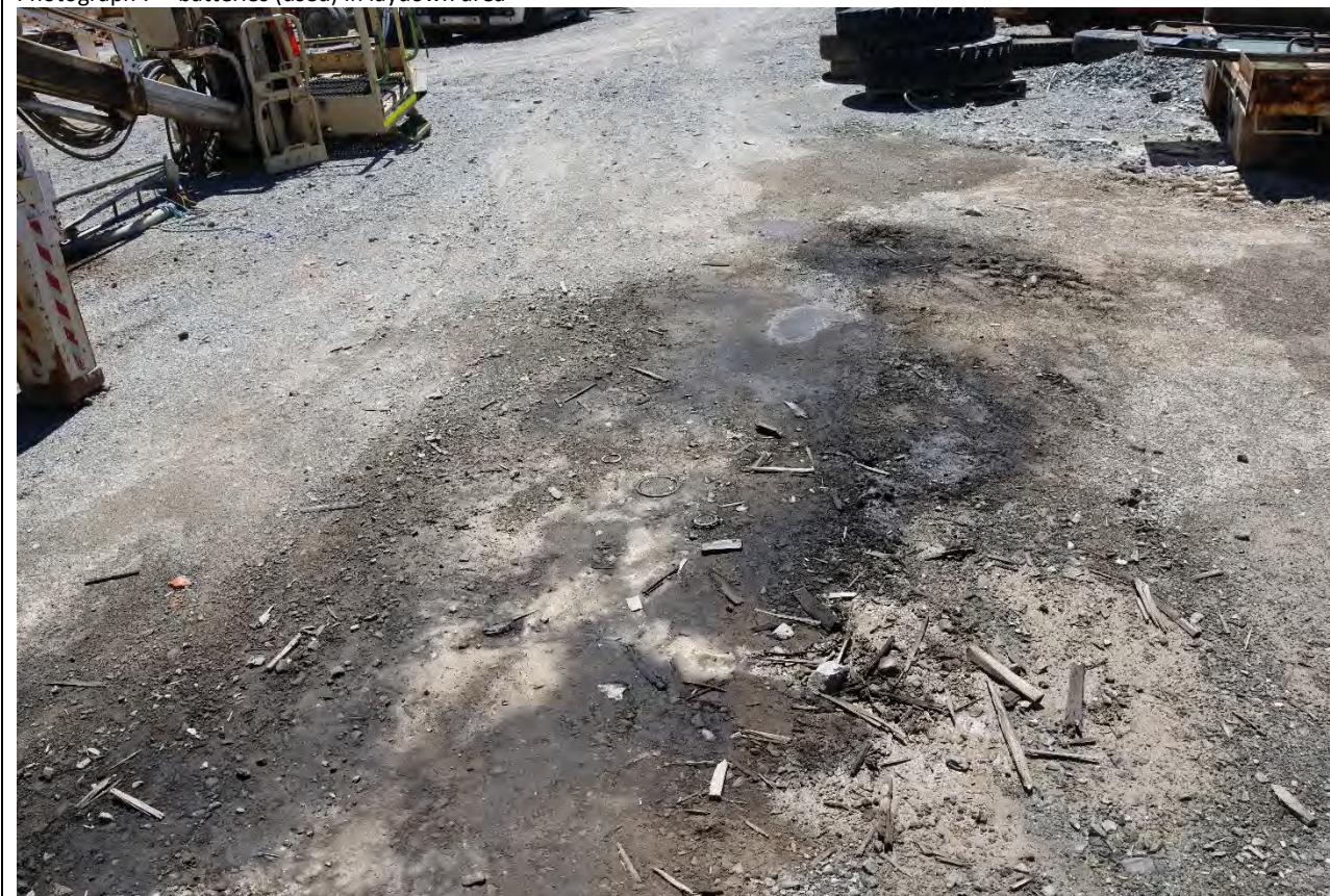
Photograph 8 – Oil contaminated soils in laydown area
