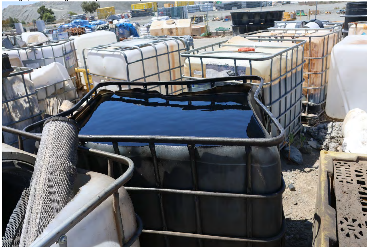
Photograph 10 – Waste oil and other waste liquids, uncontained in laydown area
