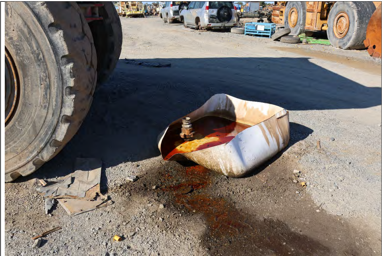
Photograph 9 – Waste Oil (drained from derelict plant) and soil contamination
